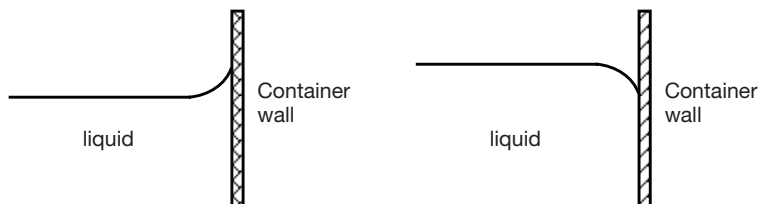
FIGURE 4.28 Figure showing that the surface of liquids acting like membranes due to unbalanced forces
